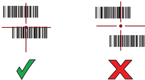
Figure 3-7 Imager Pick List Mode with Multiple Bar Codes - Standard Range
