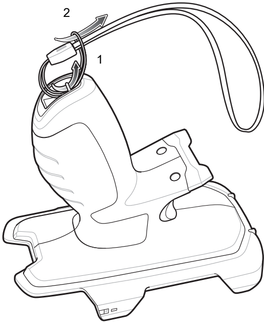
Figure 106 Install Attachment Plate to Handle
