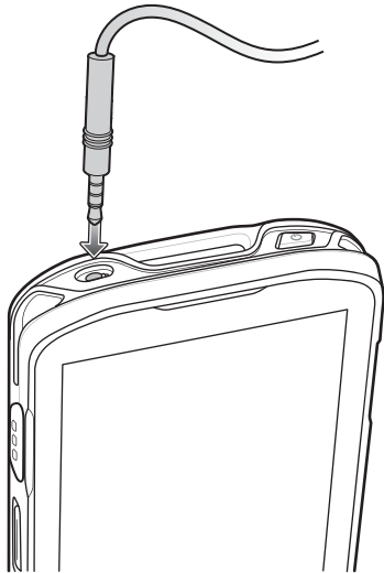
Figure 103 Audio Adapter Installation
