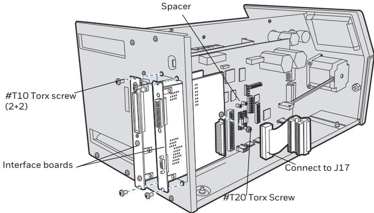
13. Installation of one board: Attach the interface board in the innermost slot in the printer's rear plate using the two screws left over when you removed the original cover plate. Using the #T20 Torx screw you previously removed, attach the interface board to the hexagonal spacer at the center of the CPU board.
