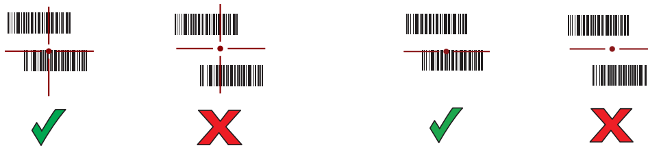
Figure 99 Pick List Mode with Multiple Barcodes in Aiming Pattern: Standard and Extended Range
