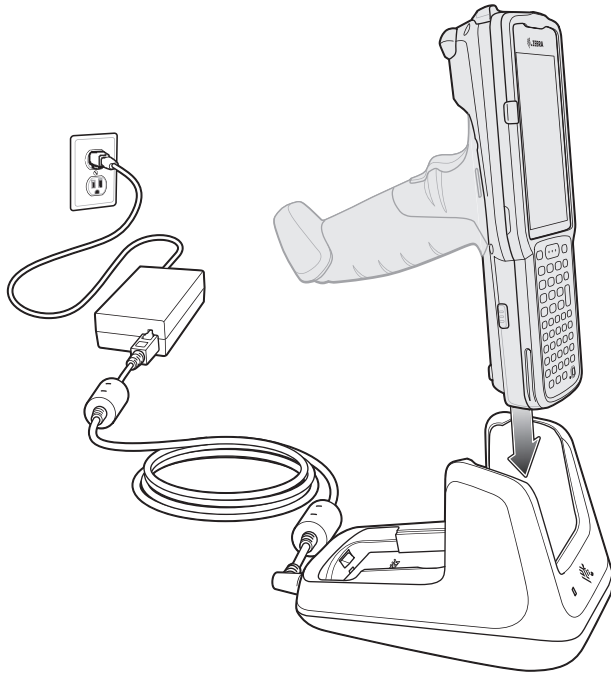
Figure 11 MC33XX Battery Charging
