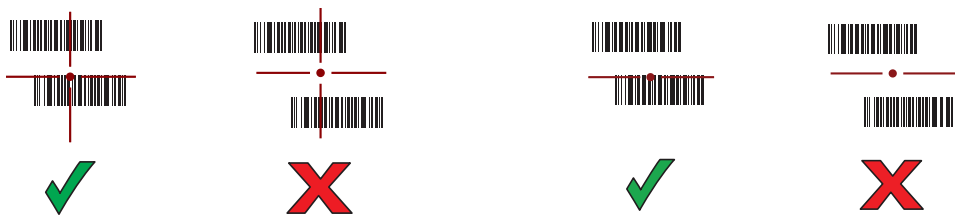
Figure 96 Pick List Mode with Multiple Barcodes in Aiming Pattern: Standard and Extended Range
