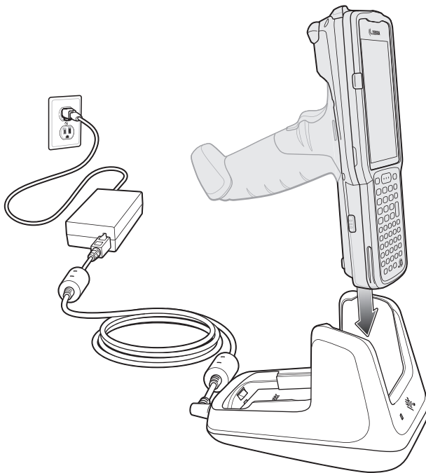
Figure 118 MC33XX Battery Charging
